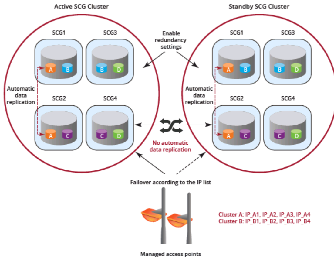
FIGURE 54 Cluster Redundancy for Active-Standby Mode
