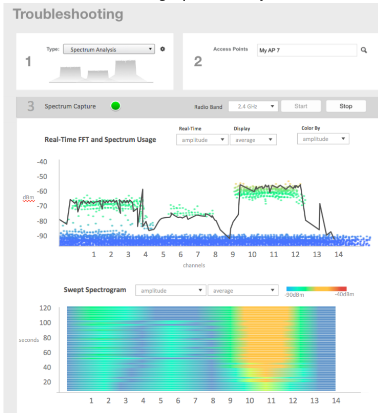
FIGURE 126 Troubleshooting - Spectrum Analysis
